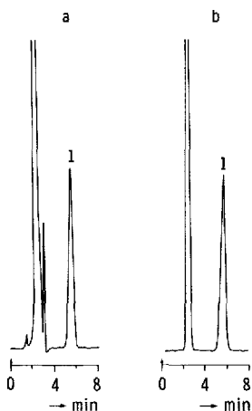
Fig. 3. Determination of lactose (1) in skim-milk. a, 10- \mu\text{l} injection of a Biggs filtrate (RI, \times 16 ); b, 40- \mu\text{l} injection of an acetate-acetonitrile filtrate (RI, \times 8 ). Column: LiChrosorb-DIOL. Eluent: acetonitrile-water (80:20). Column temperature: 35°C. Flow-rate 1.5 ml/min.
